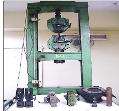
Figure 1: Tensile testing machine with jaws and fixtures
