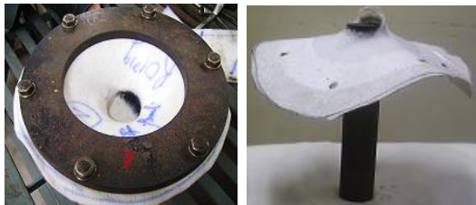
Figure 3: CBR test clamp setup and plunger
