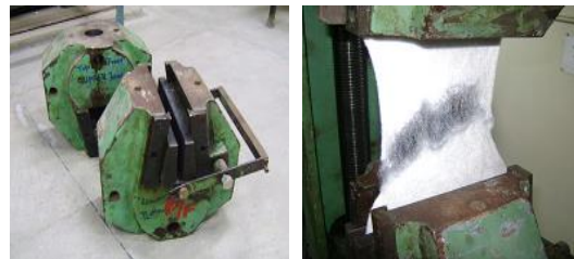
Figure 2: Wide width jaws and specimen during testing
